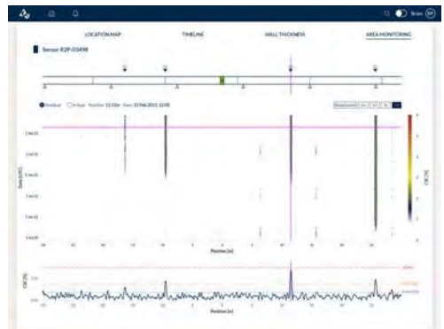
Area Monitoring data visualized on GUL Studio: Easy-to-understand pipe condition tracking.
